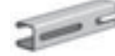
AS 520S Channel w/ Long Slots Size: 1 5/8" x 1 3/8" x 12 GA. 1 3/8" x 3" Slots on 4" Centers Page 34
