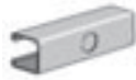
AS 300KO Channel w/ Knock Outs Size: 1 1/8" x 1 3/8" x 12 GA. 7/8" Knock Outs on 6" Centers Page 31
