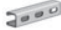
AS 500EH Channel w/ Elongated Holes Size: 1 5/8" x 1 3/8" x 14 GA. 3/8" x 1 1/8" Elongated Holes on 2" Centers Page 33
