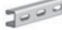
AS 560EH Channel w/ Elongated Holes Size: 1 5/8" x 1 3/8" x 16 GA. 3/8" x 1 1/8" Elongated Holes on 2" Centers Page 35
