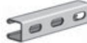
AS 500EH SS/ZD/HG Channel w/ Elongated Holes Size: 1 1/2" x 1 3/8" x 14 GA. 3/8" x 1 1/8" Elongated Holes on 2" Centers Page 88
