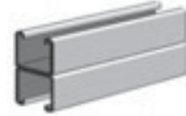
AS 200BTB EH SS/ZD/HG Welded Channel Size: 1 1/2" x 3 1/2" x 12 GA. Two Pcs. AS 200EH Welded Back-to-Back 3/8" x 1 1/8" Elongated Holes on 2" Centers Page 86
