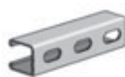
AS 210EH SS/ZD/HG Channel w/ Elongated Holes Size: 1 1/2" x 1 3/8" x 14 GA. 3/8" x 1 1/8" Elongated Holes on 2" Centers Page 87
