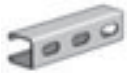
AS 300EH Channel w/ Elongated Holes Size: 1 1/8" x 1 3/8" x 12 GA. 3/8" x 1 1/8" Elongated Holes on 2" Centers Page 31
