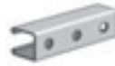
AS 300H Channel w/ Holes Size: 1 1/8" x 1 3/8" x 12 GA. 9/16" Holes on 1 7/8" Centers Page 31
